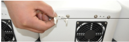
Fix the probe Holder by screw
